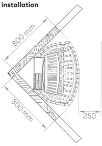
A non-combustible wall is needed on the sides of the heater.
